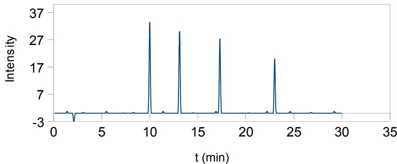
HPLC-Column: **AppliChrom OTU Amino**, 5μ, 250x4.6mm, eluent: ACN/H<sub>2</sub>O 75/25, temperature: 25°C, flow: 1ml/min, detection: RI (alternative ELSD), Peaks in elution order: **Fructose, Glucose, Sucrose, Maltose**.
