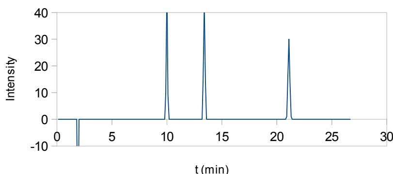
HPLC-Column: **AppliChrom OTU Amino**, 5µ, 250x4.6mm, eluent: ACN/H<sub>2</sub>O 85/15, temperature: 27°C, flow: 1ml/min, detection: RI (alternative ELSD), Peaks in elution order: meso-Erythritol, Xylitol, Sorbitol.
