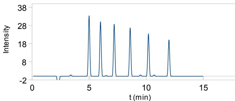
HPLC-Column: **AppliChrom OTU Amino**, 5μ, 250x4.6mm, eluent: ACN/H<sub>2</sub>O 55/45, temperature: 27°C, flow: 1ml/min, detection: RI (alternative ELSD), Peaks in elution order: Maltose, Maltotriose, Maltotetraose, Maltopentose, Maltohexose, Maltoheptose
